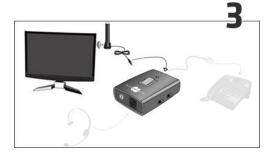
Insert the cord for the Busylight lamp into the Busylight box and mount the lamp on your screen (or another visible place) with the round tape. Avoid placing the lamp in direct sunlight.
