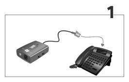
Take the headset cord out of the telephone and insert the pre-installed cord from the Busylight box into the telephone instead.
